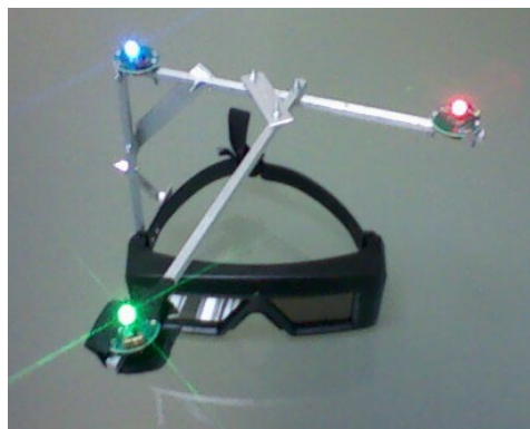
Figure 4.2. LEDs mounted on a frame attached to stereo goggles
