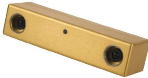
Figure 4.3. Stereo camera that is being used by RWB.
