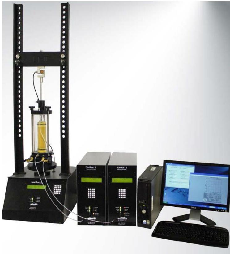
Figure.3.8. Automatic triaxial system
