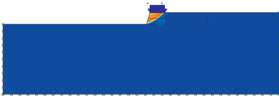
Figure 4.20. Terzaghi's Bearing Capacity Mechanism with Slope Failure.
