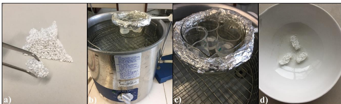
Figure 3.8. Wash coating preparation system. a) commercial ceramic foam, b-c) wash coating under ultrasonic mixing, d) obtained coated monoliths
