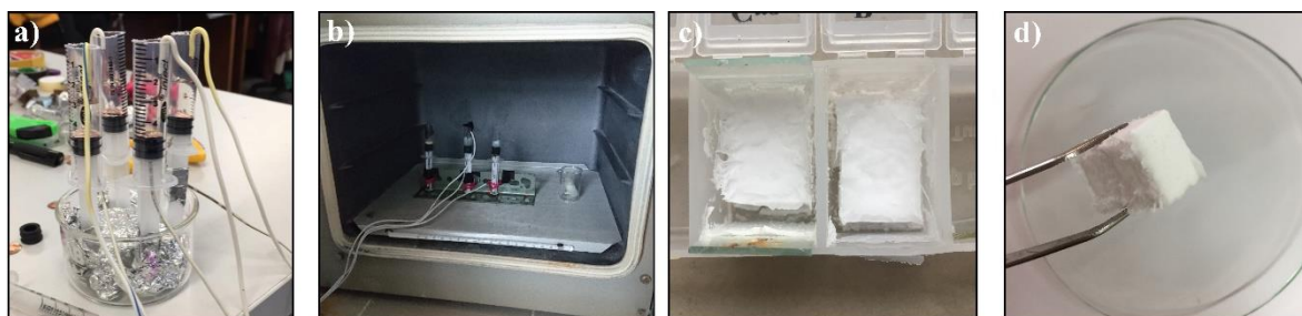
Figure 3.6. Different systems for sol-gel preparation under electric field. a) system with using copper plates, b) with Pt-coated copper plates, c) ITO coated glass plates, d) synthesized catalyst with using ITO coated glass plates
