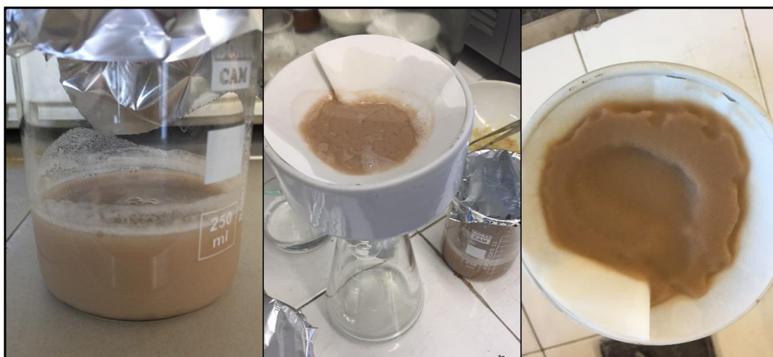
Figure 3.3. Preparation steps of Mn-SiO 2 support. a) slurry after oven b) during filtration, c) after filtration
