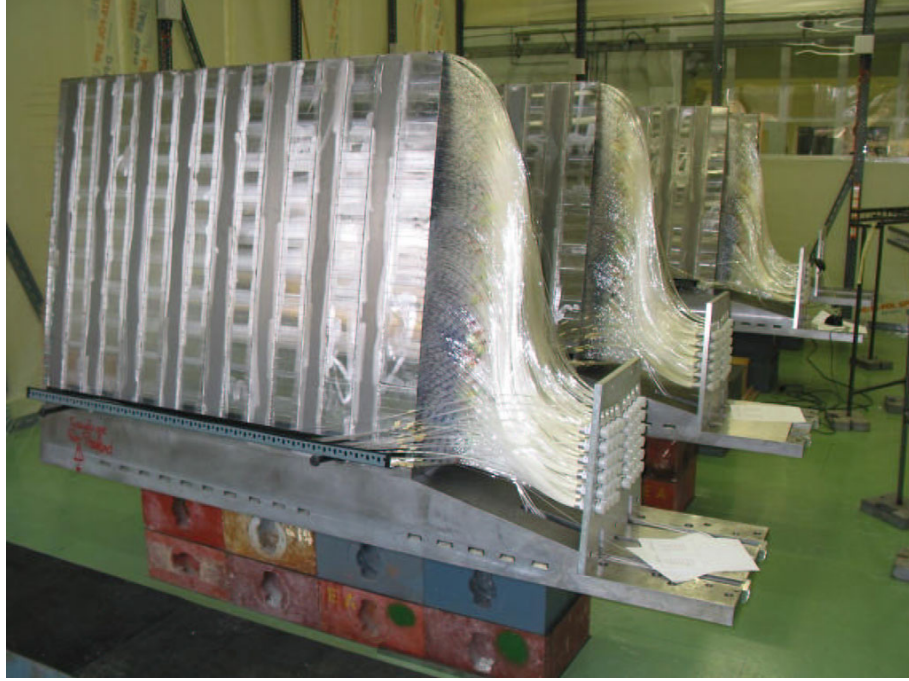
Figure 4.1. A picture of HF wedges where the quartz fibers emerging from the back of the wedge can be seen.
