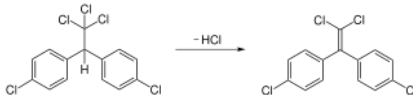
(b) Degradation of DDT to form DDE by an elimination of HCl
