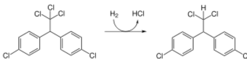
(a) Reductive dechlorination of DDT to form DDD
