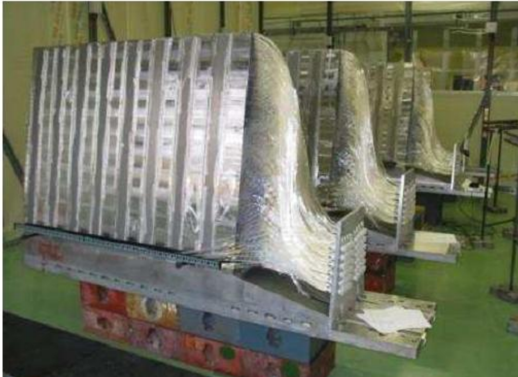
Figure 5.2. HF wedges with fibers inserted into the steel absorber
