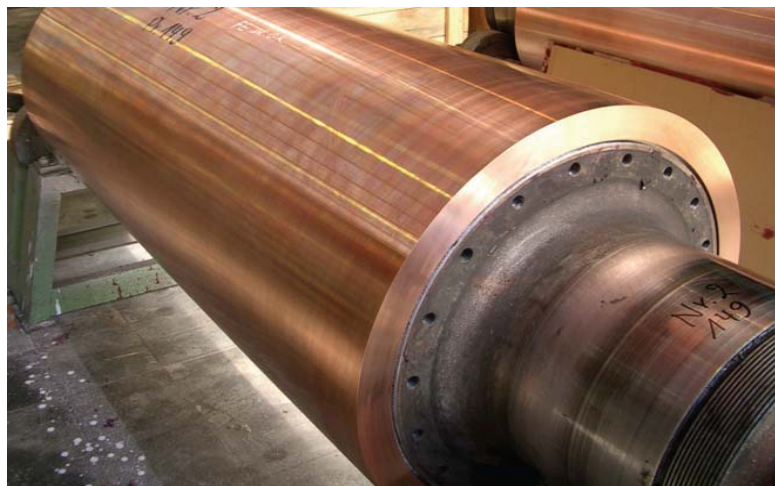
Figure 2.21. Twin roll casting roll with copper shell [25]
