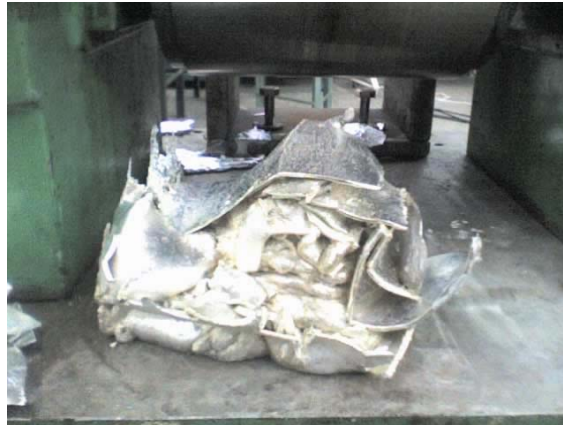
Figure 4.5. Result of casting trials in casting speed of 12.5m/min
