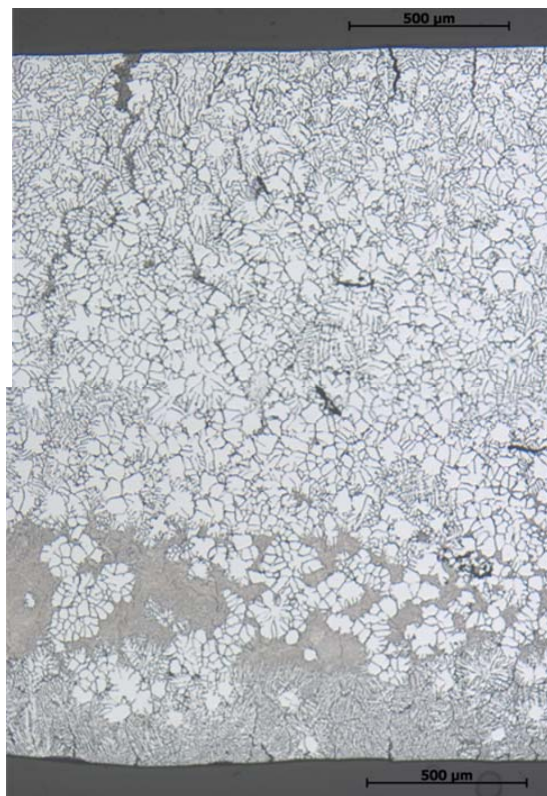
Figure 4.12. Second phase particles of experimentally cast AA1050 modified with Mg+Mn
