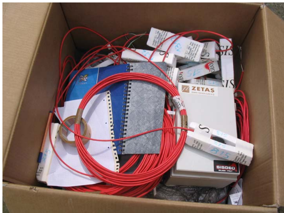
Figure 4.7. Strain gauges with supplied specific length cables
