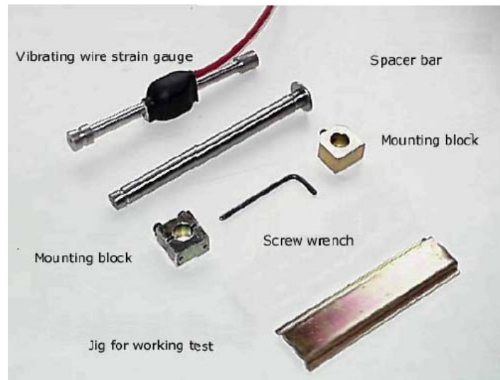
Figure 4.2. Vibrating wire strain gauge for surface accessories
