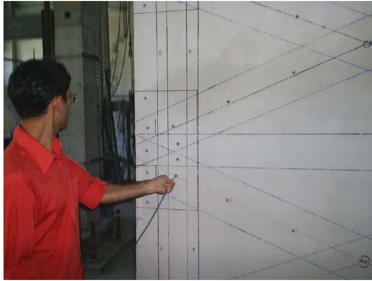
Figure 3.10. Cleaning of the anchor holes
