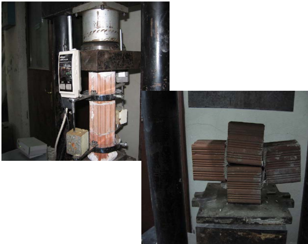
Figure 3.4. Test set-up for compressive and shear strengths of a masonry subassembly
