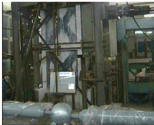
Figure 4.13. Cracking planes at different elevations during the failure of the specimen
