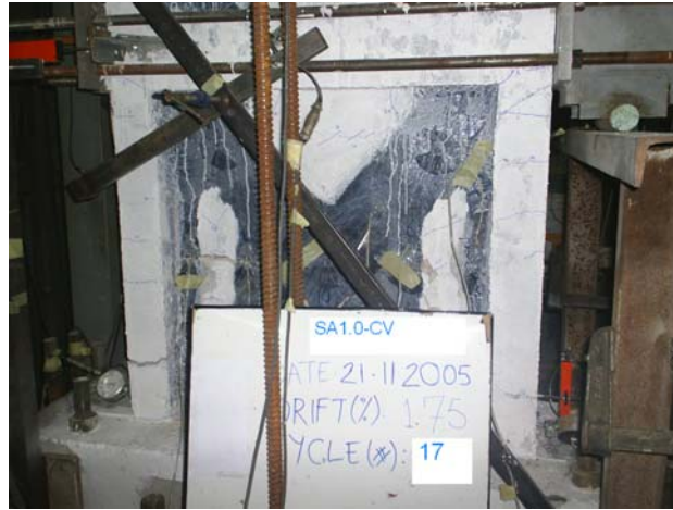
Figure 4.11. Specimen SA1.0-CV at the end of the test
