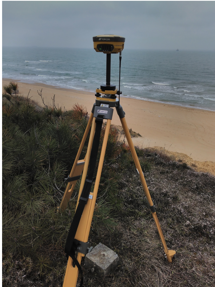
Figure 2.1. Base GNSS receiver, March 24, 2017 (preparation survey).
