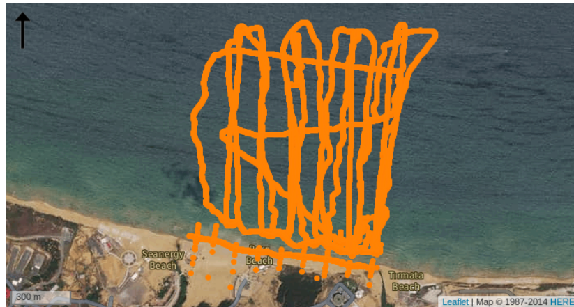
Figure 2.5. Point distribution from March 2017 survey, 13,347 usable data points.
