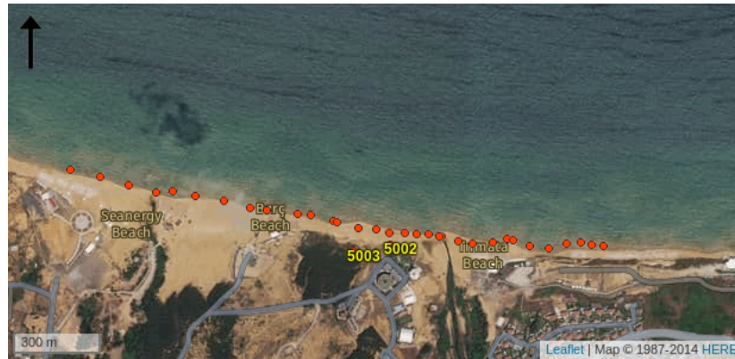
Figure 2.9. Shoreline and benchmark locations measured with GPS on June 14, 2001.
