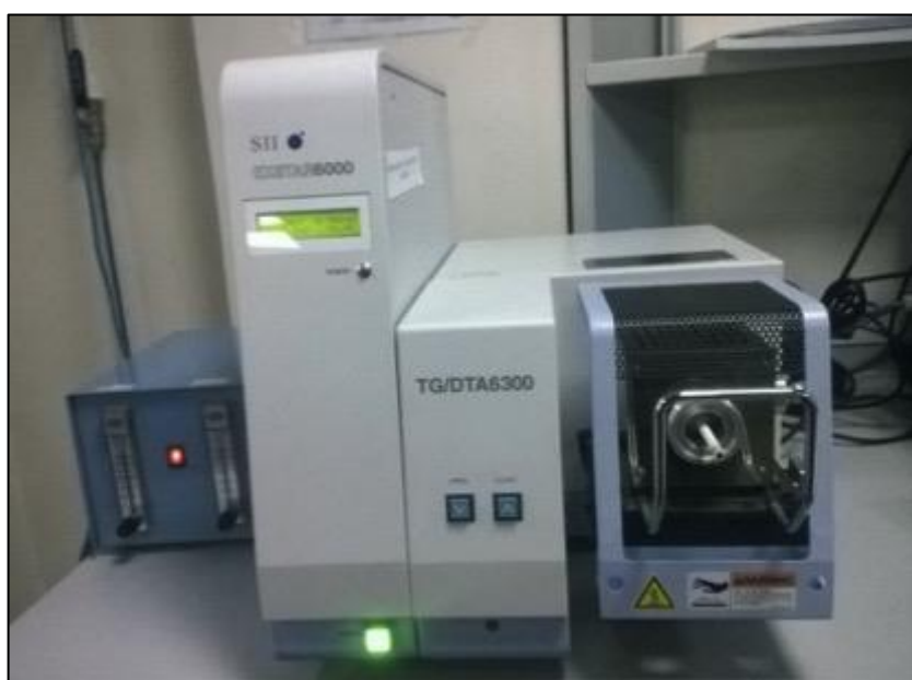
Figure 3.18. EXSTAR SII TG/DTA6300 Analyzer
