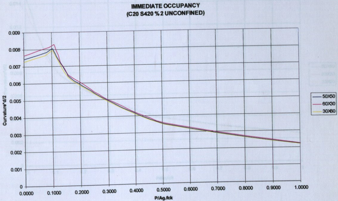
Figure 2.7. Effects of section dimensions for unconfined sections
