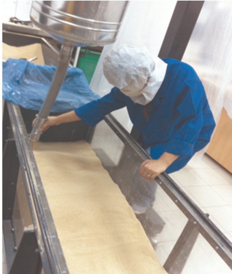
Figure 4.7. The new pluviation system.
