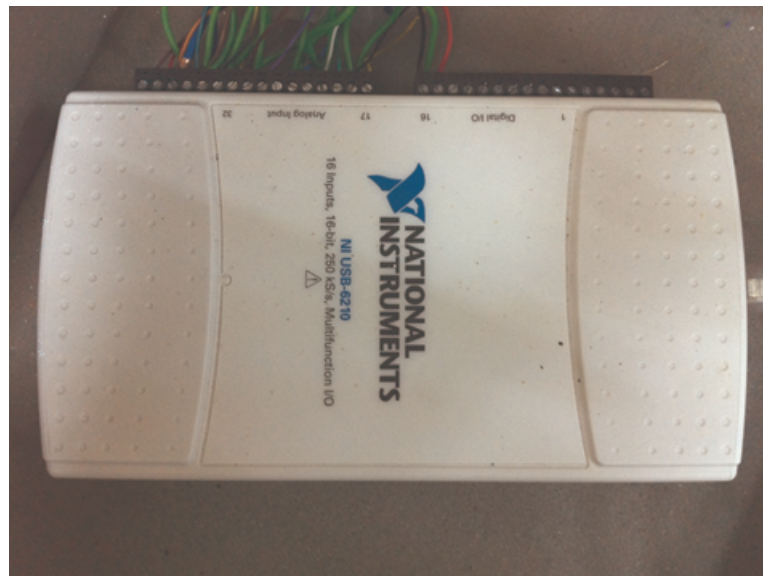
Figure 4.5. The data acquisition system of LabVIEW.
