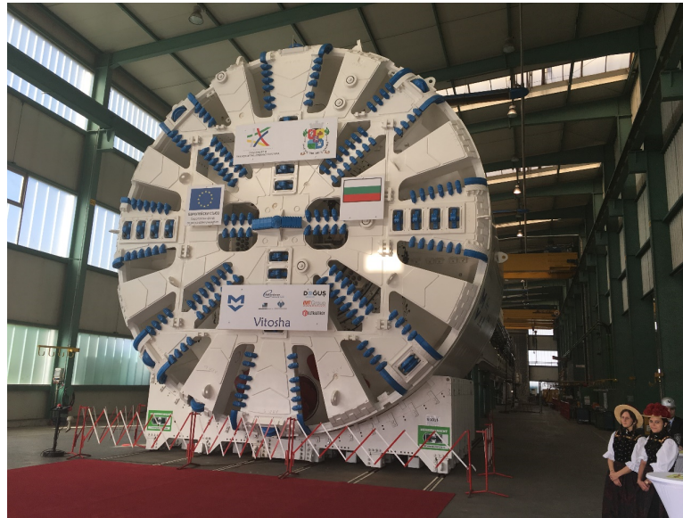
Figure 5.11. EPB TBM Cutterhead used in the Project.
