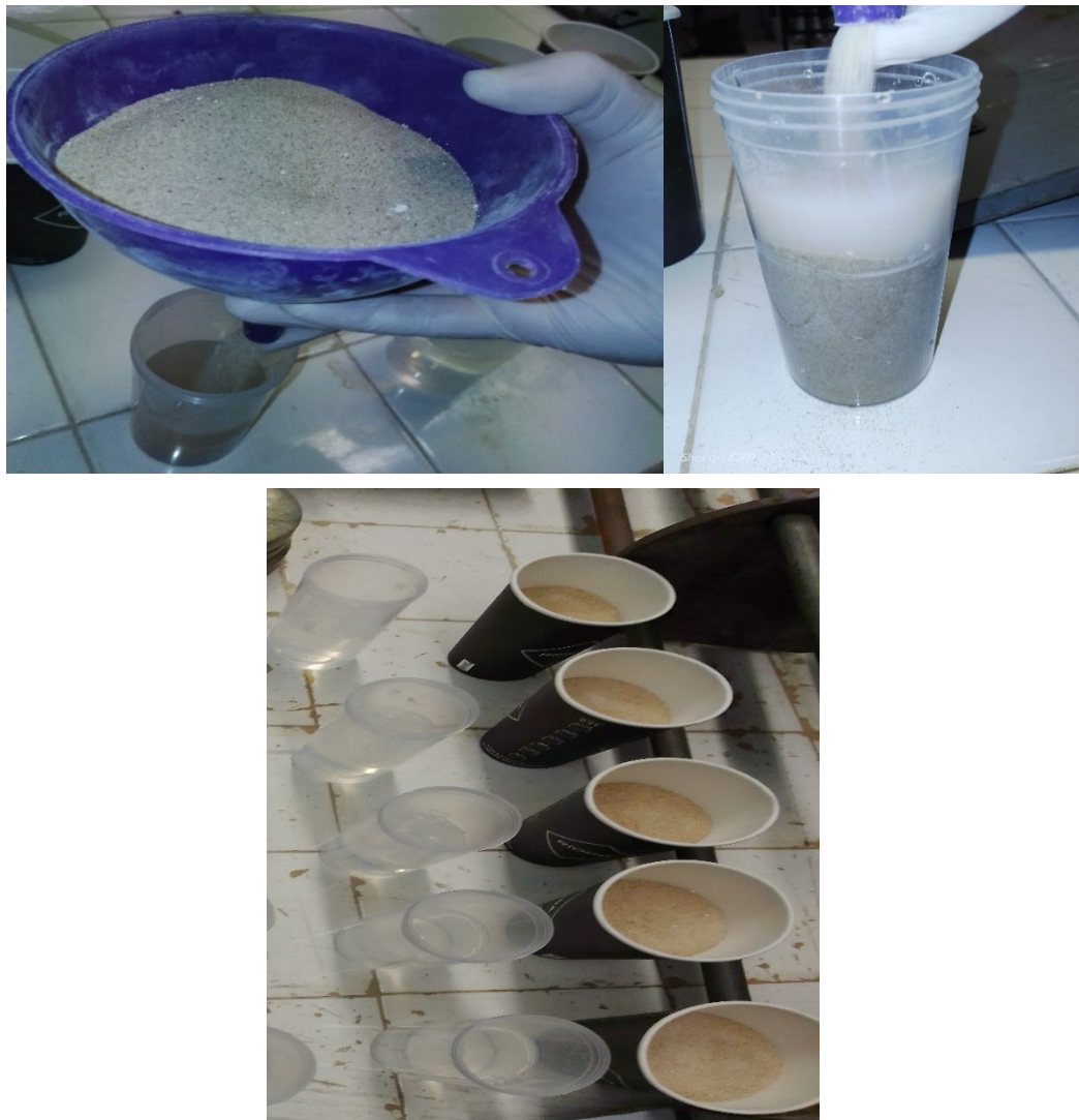
Figure 5.13. Preparation of components and pluviation of sand-MgO blends into 137 mL water by funnel at certain height with spiral motion.
