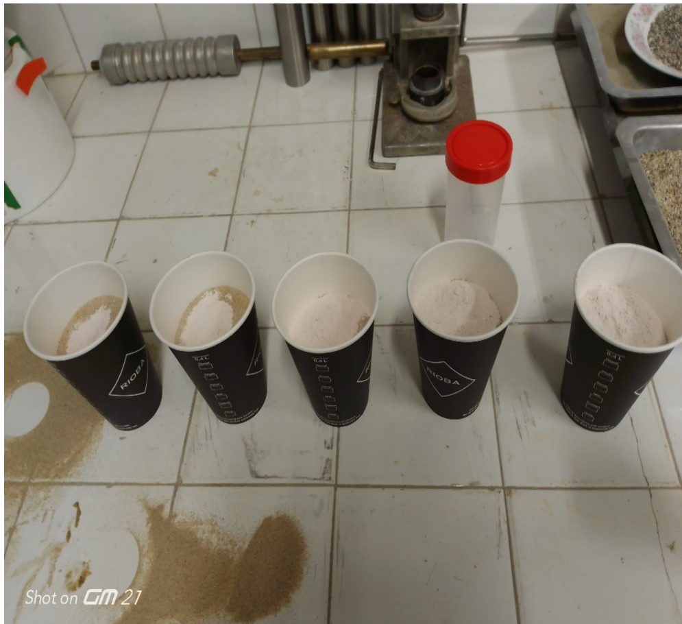
Figure 5.11. Dry Mixture of Sand-MgO before blending.
