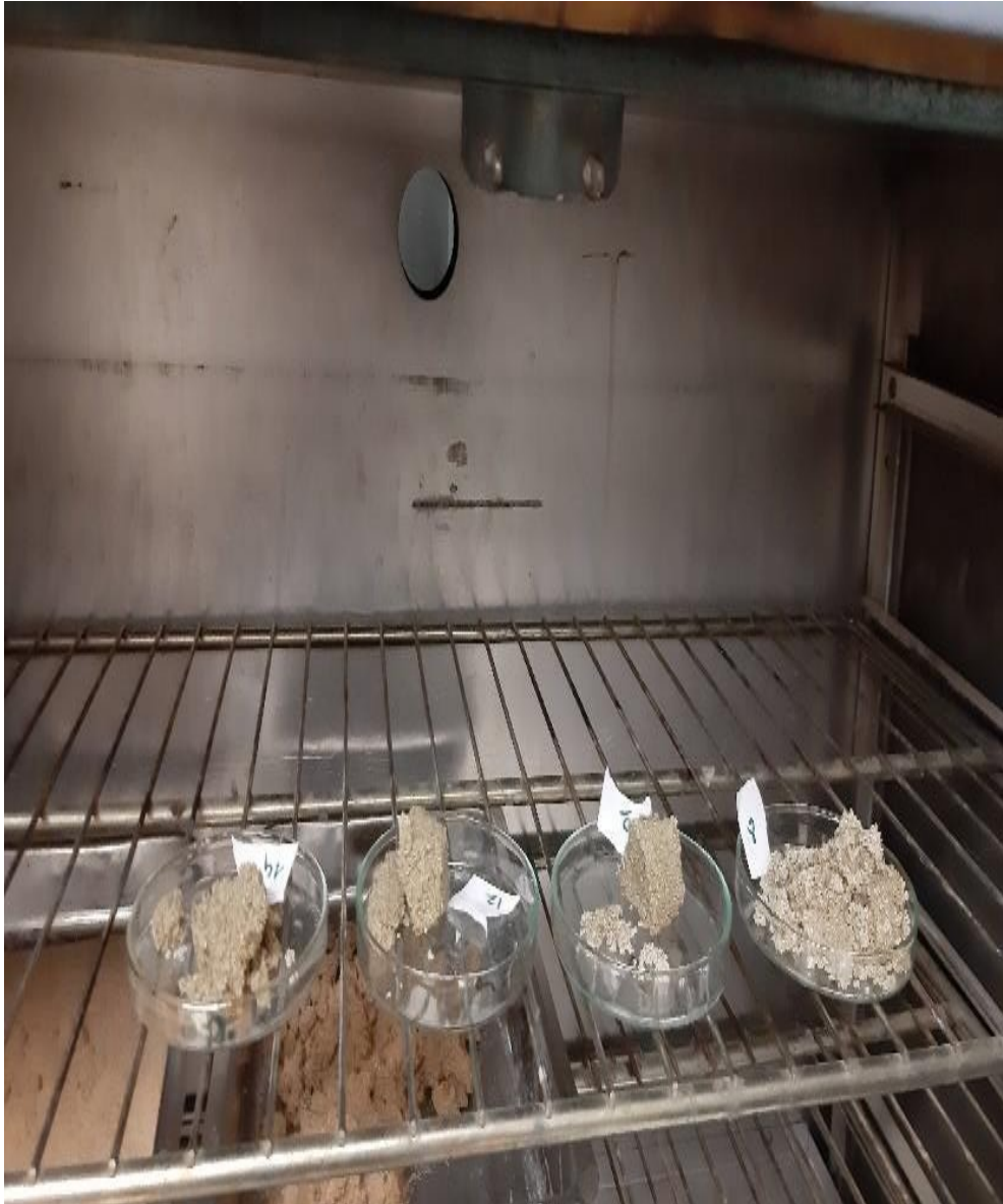
Figure 5.20. Determination of water content of samples after experiment.
