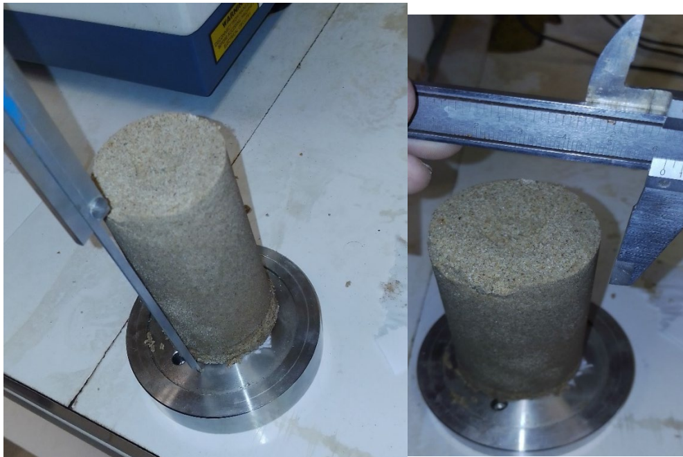
Figure 5.16. Measurement of dimension of improved samples after curing periods.
