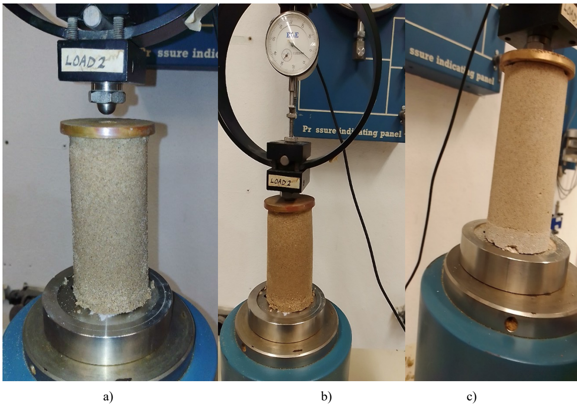
Figure 5.18. Placement of specimen into LDVT Frame : a) 0.5% MgO Sample for 7 days, b) 2% MgO Sample for 3-days, c) 4% MgO Sample for 14-days.
