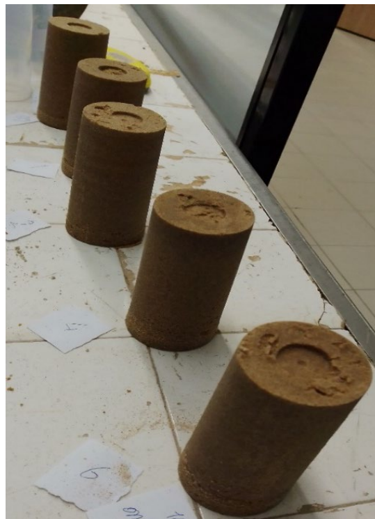
Figure 5.15. Samples cured for 3,7 and 14 days under laboratory condition after extracted from mould after 2 day.
