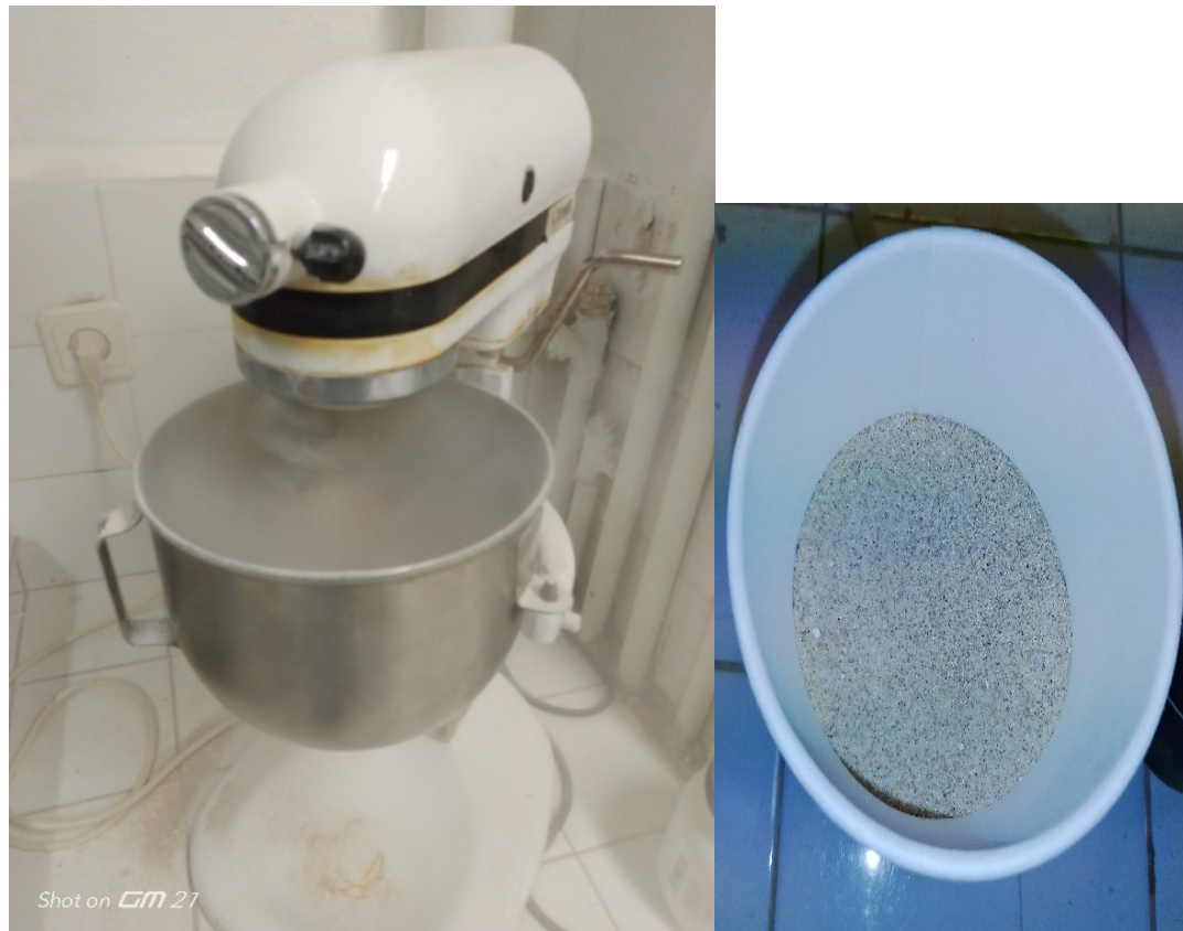
Figure 5.12. Dry mixture of sand and magnesium oxide after 10 minutes blending.
