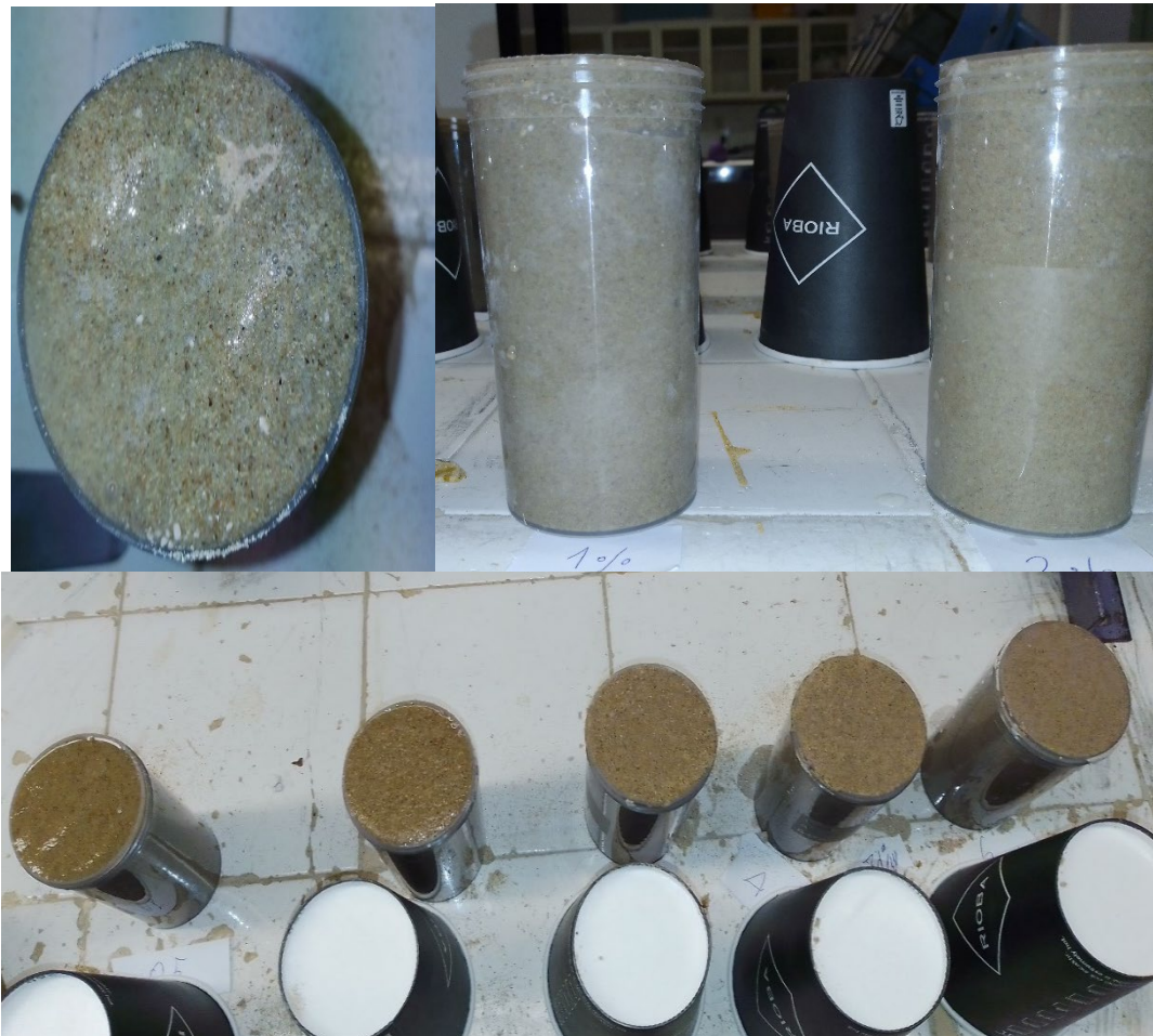
Figure 5.14. The moulding of samples after pluviation of dry blends into water and check for fully- saturation, excess components and remoulded water content.
