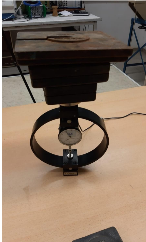
Figure 5.17. Calibration of Load Gauge by putting surcharges with increasing rate.
