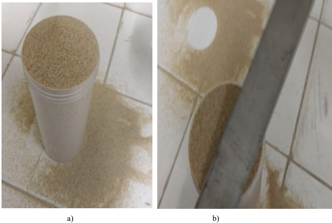
Figure 5.7. The determination of bulk density and void ratio under laboratory conditions : a) Filling the plastic mould with dry sand completely, b) Trimming of excess dry soil.
