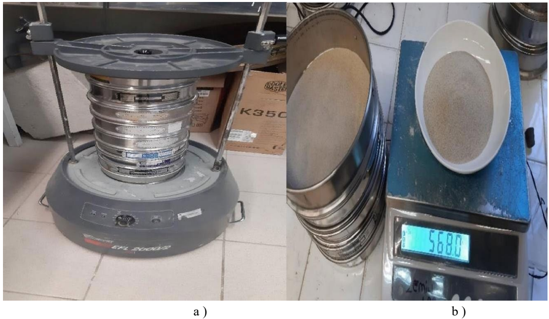
Figure 5.4. Grain Size Distribution Test for pure sand : a) Sieving , b) Weighing.
