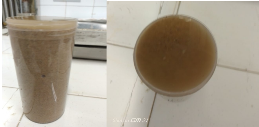
Figure 5.9. Saturation check for 400.84 g dry sand pluviated into 137 mL water within plastic cylindrical mould.
