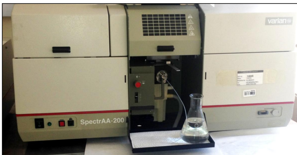
Figure 3.1. Varian Spectra AA-200 model of flame atomic emission spectroscopy.
