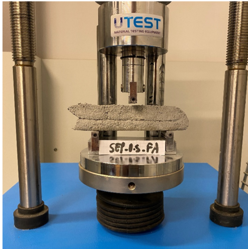
Figure 2.18. 3-Point bending test setup.
