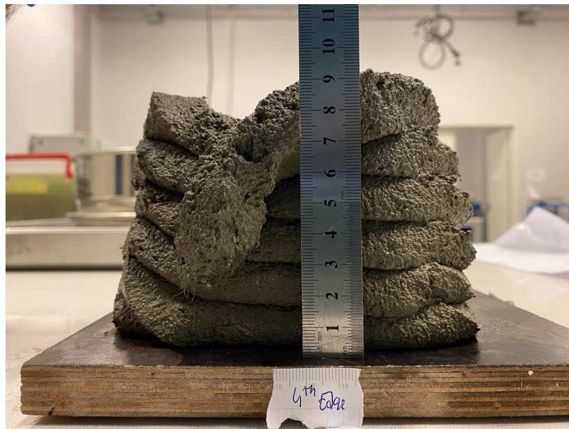
Figure 3.14. Failure of the structure during printing of the 6 th layer.
