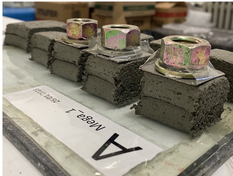
Figure 2.12. Loading additional weight on top of the samples of interlayer bonding test.
