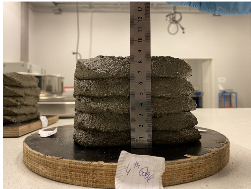
Figure 2.8. Measuring the height of the printed specimen for stability test.
