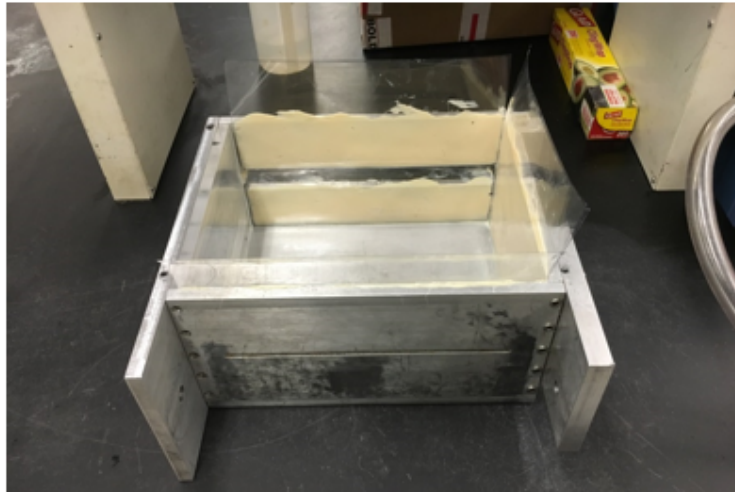
Figure 3.14. Gridded Latex Membrane 0.15 mm.
