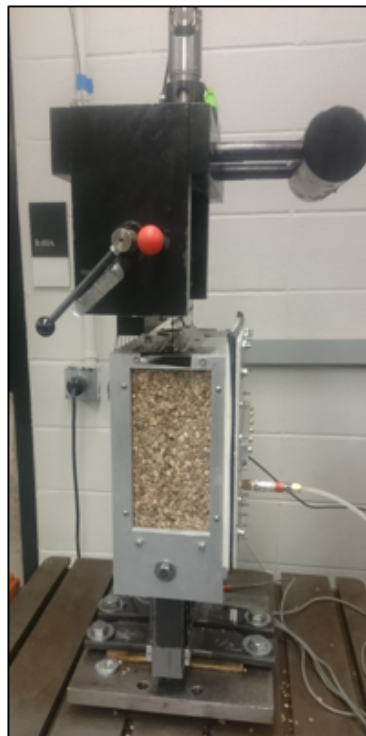
Figure 3.10. Modified Small Pullout Test Setup.
