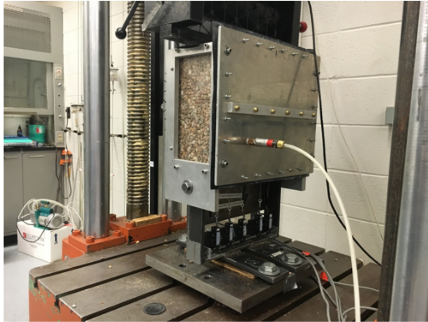
Figure 3.19. Small Pullout Test Final Setup.
