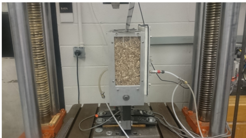
Figure 3.8. Trial Test with 2 Pressurized Air Bladders and 7.5 cm sleeve.
