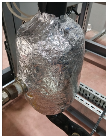
Figure 4.15. Installed liquid collector on ORC test rig.
