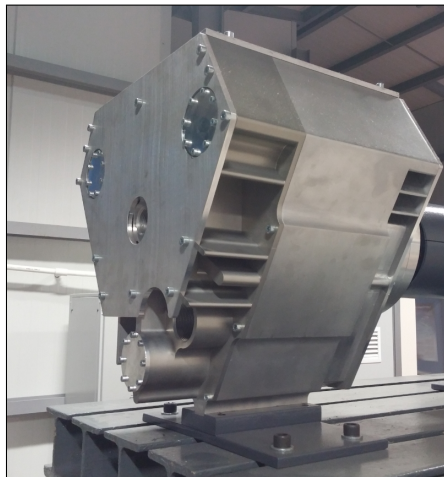
Figure 4.2. Installed scroll type expander on ORC test rig.
