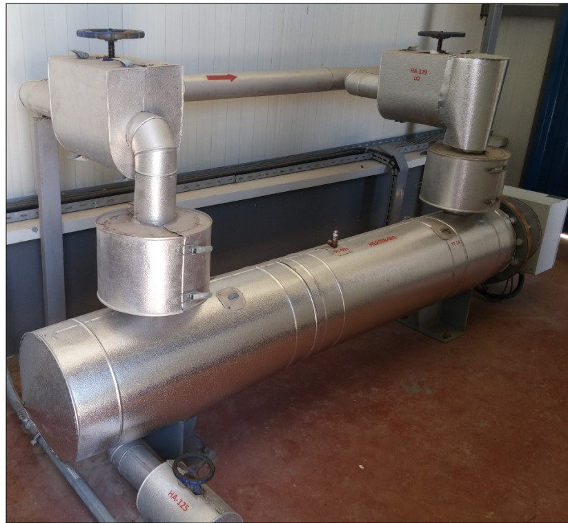
Figure 4.10. Installed heater on ORC test rig.
