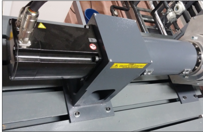
Figure 4.14. Installed dynamometer on ORC test rig.
