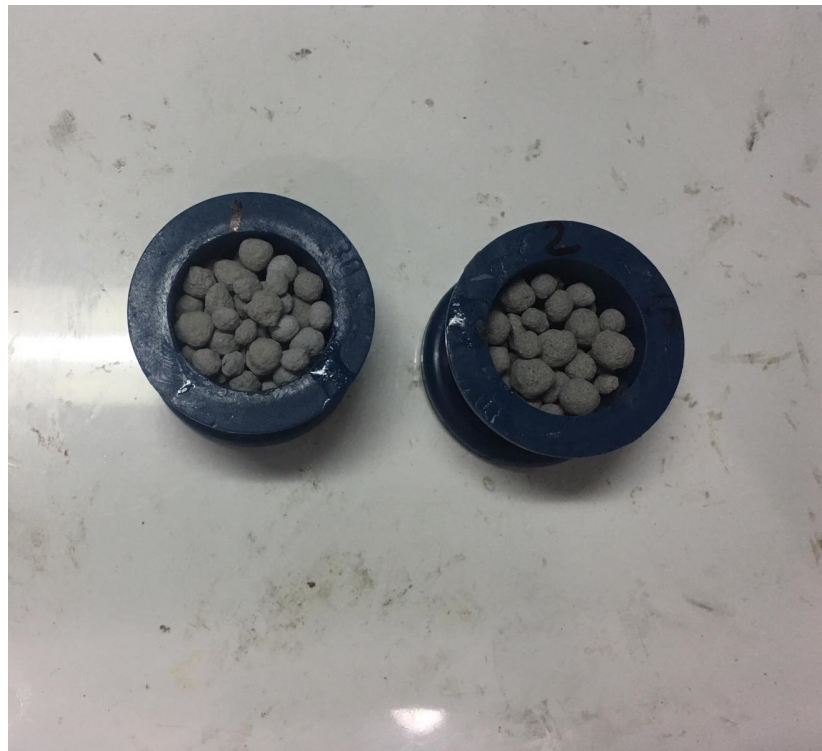
Figure 3.16. Sample preparation for thin section analysis
