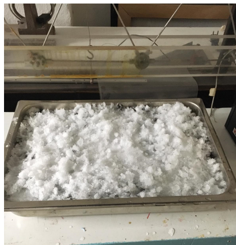
Figure 3.3. Fly ash samples with snow addition at the beginning of freezing cycle
