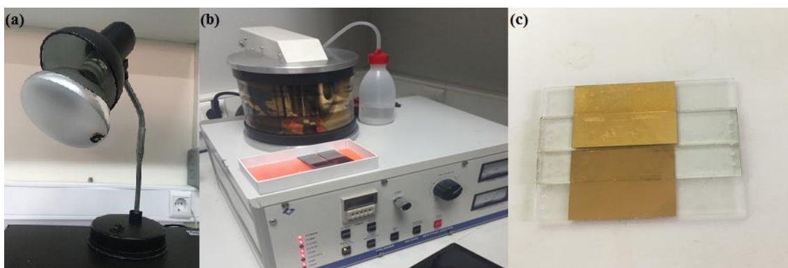
Figure 3.5. (a) The UV light source (b) the sputtering device. (c) The microchannel with glass slides coated with gold.
