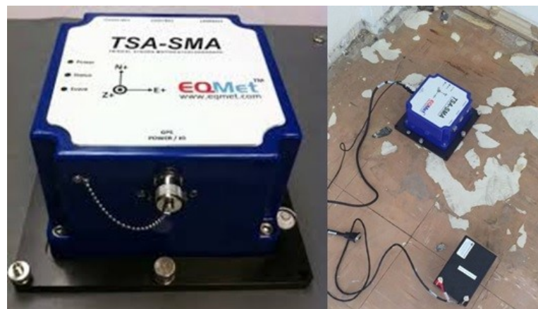
Figure 3.1. Kinemetrics TSA-SMA triaxial accelerometer used in AVT.
