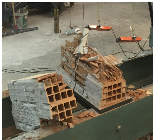
Figure 4.6. Brittle failure of the partition wall specimen.
