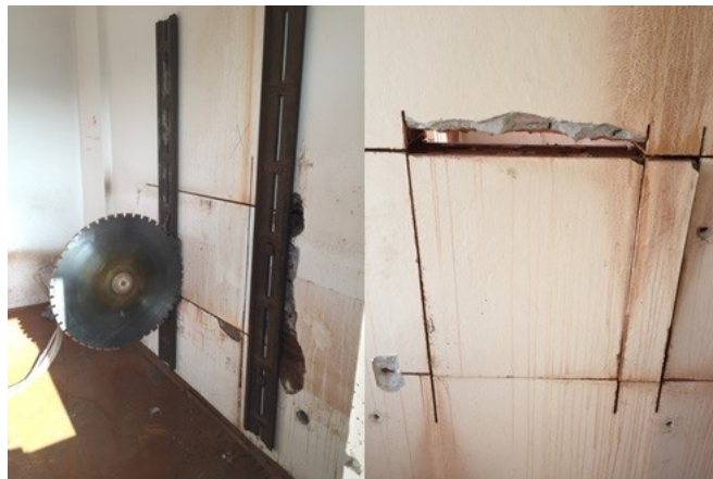
Figure 4.1. Extraction of compression and shear test specimens by sawing.
