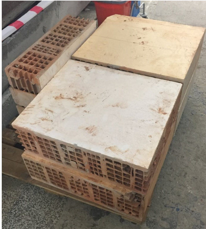
Figure 4.2. Compression and shear test specimens extracted from the building.
