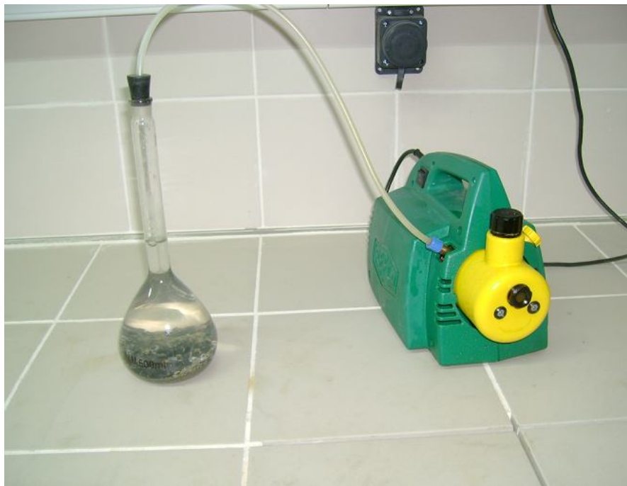
Figure 5.12 Pycnometer and vacuum pump used in the tests
