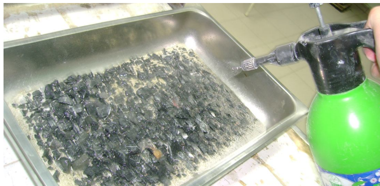
Figure 5.6. Addition of water to the aggregate mixture with a spray bottle
