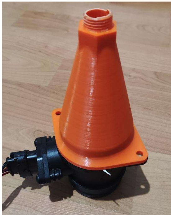
Figure 3.12. MAF Sensor with 3D Printed Connector.
