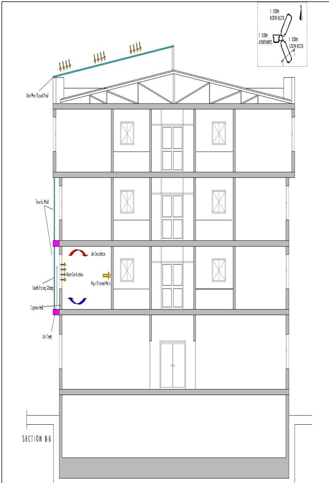
Figure 2.19. Trombe Wall Application – Building Section.
