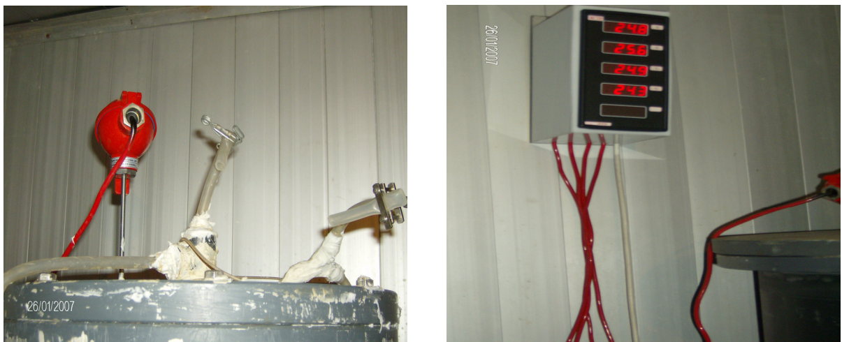
Figure 4.5. Thermocouple and temperature reading
