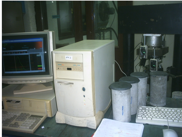
Figure 3.3. Data acquisition system of cyclic loading
