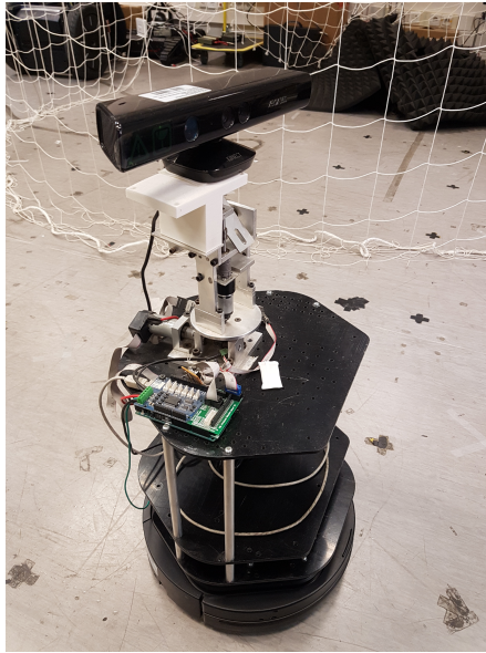
Figure 2.6. Kobuki turtlebot with pan-tilt camera
