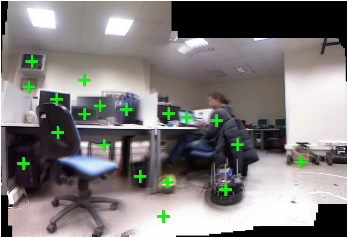
Figure 2.1. With the proposed approach, the robot couples visual exploitation and exploration. In this example, the robot has determined 19 object candidates (green crosses) after exploiting the incoming 136 frames that are acquired through 15 camera movements. The figure is obtained after stitching 15 frames with roughly 95^\circ pan and 35^\circ tilt coverage.
