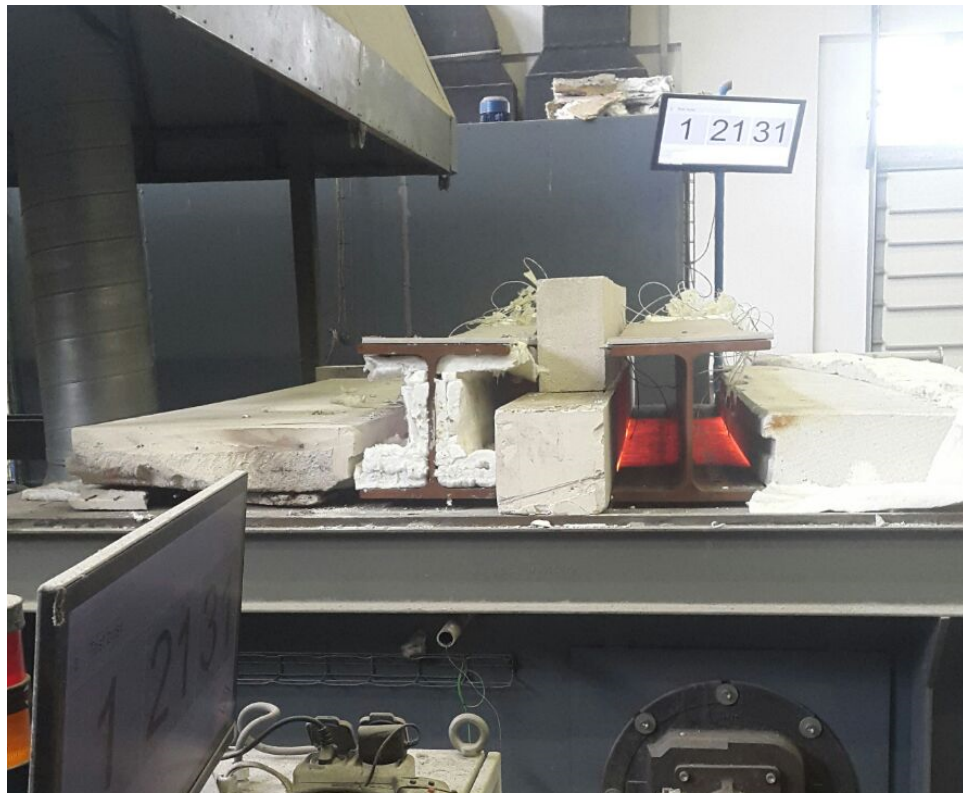
Figure 5.35. Section View during the Test for HEB 300 (80 th Minute).
