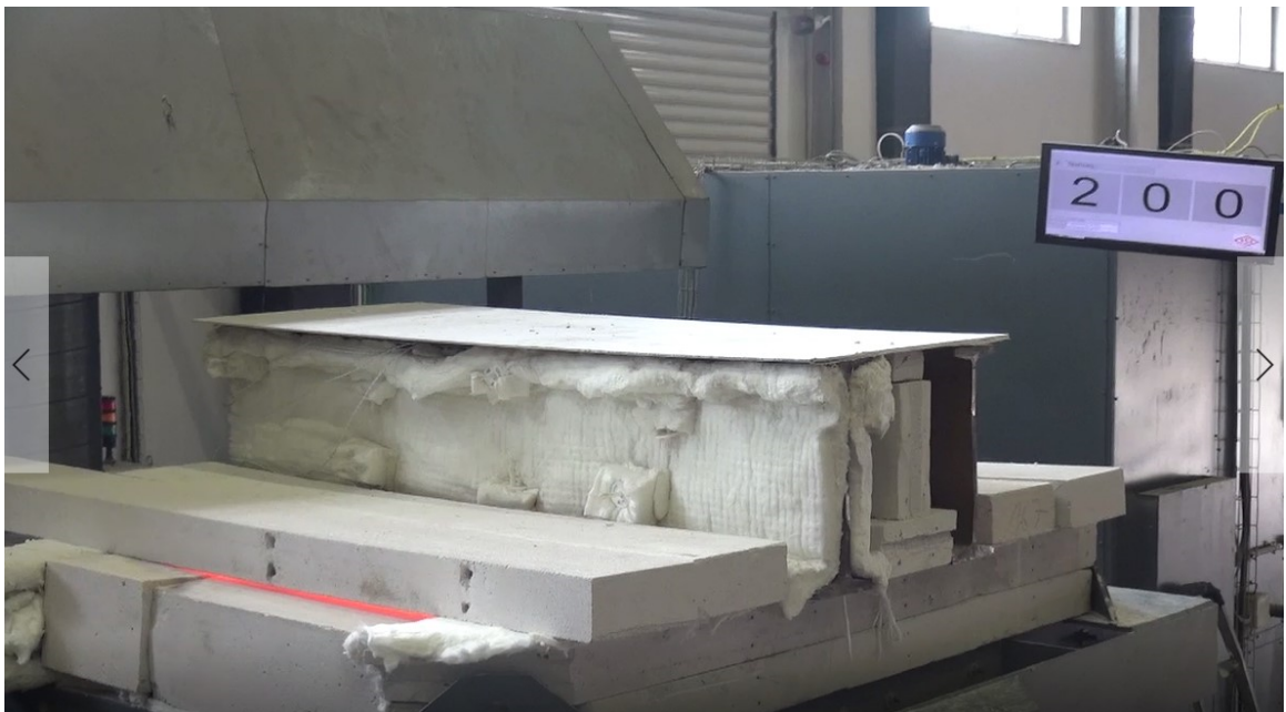
Figure 5.13. During the Test for INP 400 (120 th Minute).
