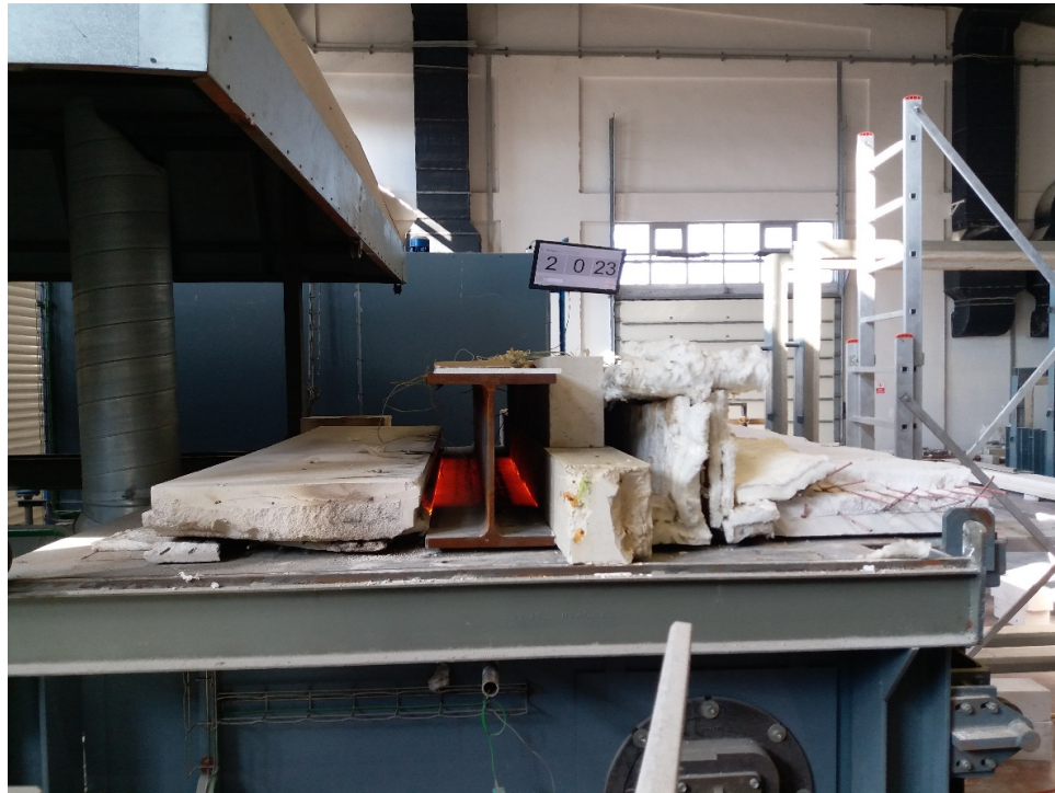
Figure 5.24. Section View at the End Of The Test For HEB 400 (120 th Minute).
