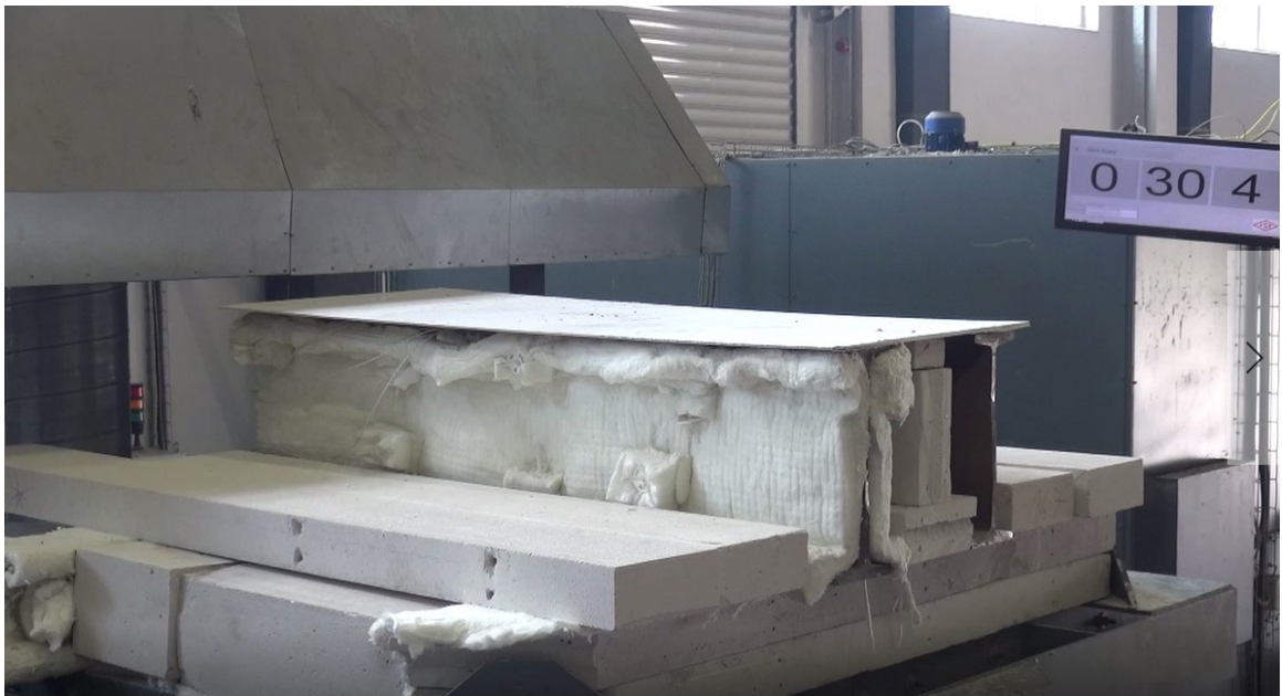
Figure 5.11. During the Test for INP 400 (30 th Minute).
