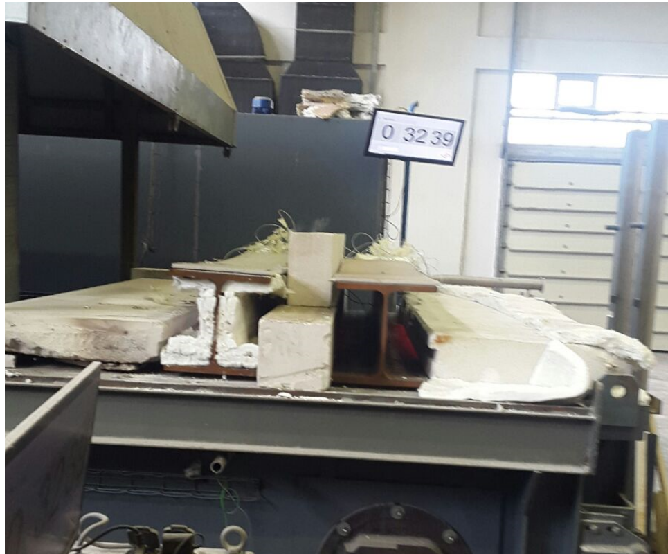
Figure 5.33. Section View during the Test for HEB 300 (32 nd Minute).
