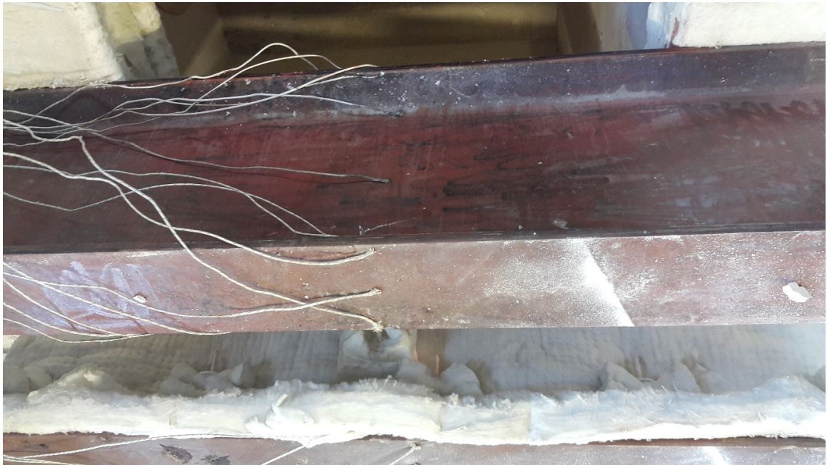
Figure 5.8. Fixed Thermocouples for INP 400.
