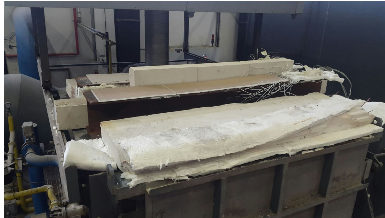
Figure 5.31. General View before the Test for HEB 300.
