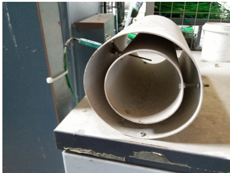
Figure 3.9. TSE Ambient Temperature Measuring Device.
