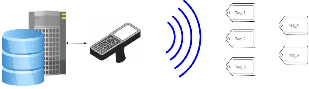
Figure 1.1. A typical RFID system
