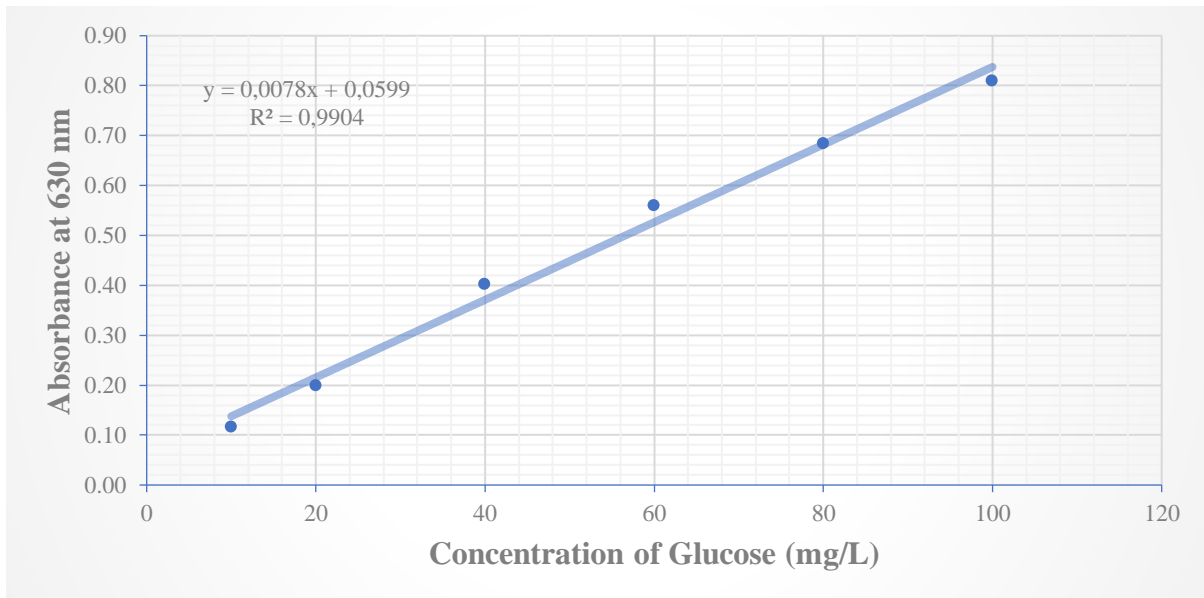
Figure A.2. Calibration curve of glucose by Anthrone method for carbohydrate analysis.
