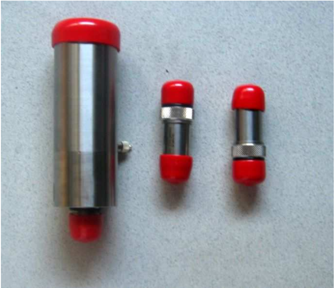
Figure 1.8. Transducers of 50 MHz, 10 MHz and 3.5 MHz.
