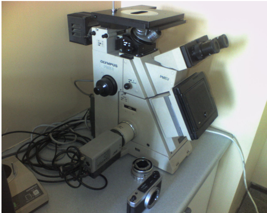
Figure 3.23. View of the Olympus microscope used for microstructural observation of the specimens
