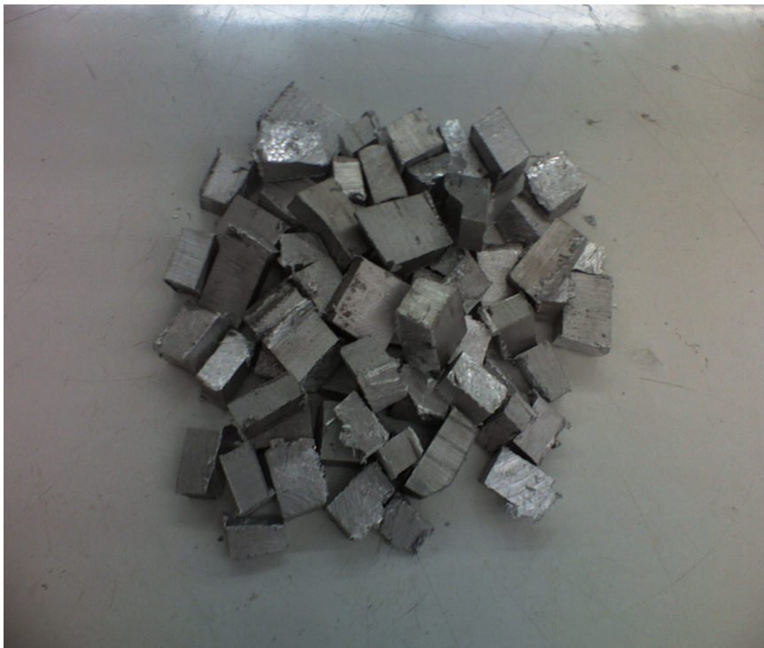
Figure 3.5. Sliced aluminum pieces using a Bosch spiral saw
