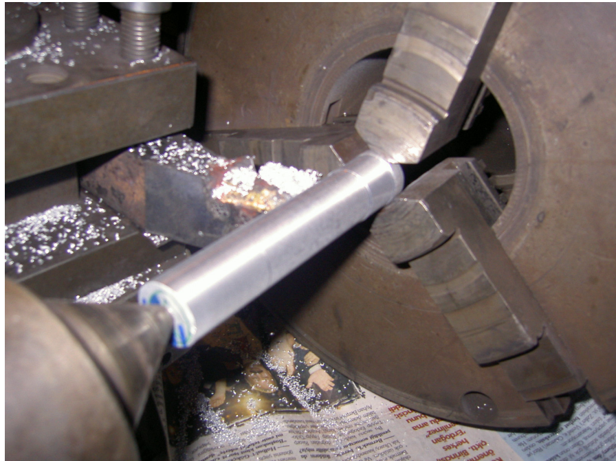
Figure 3.17. A view of turning operation and collection of chips
