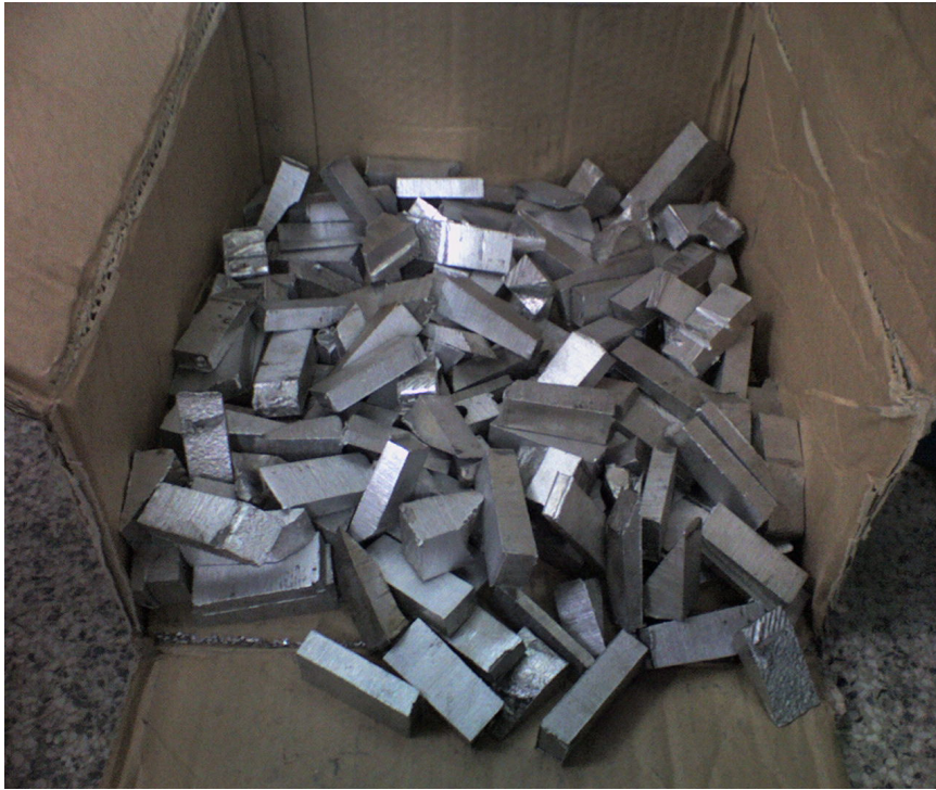
Figure 3.4. Long aluminum pieces after slicing with an Uza saw
