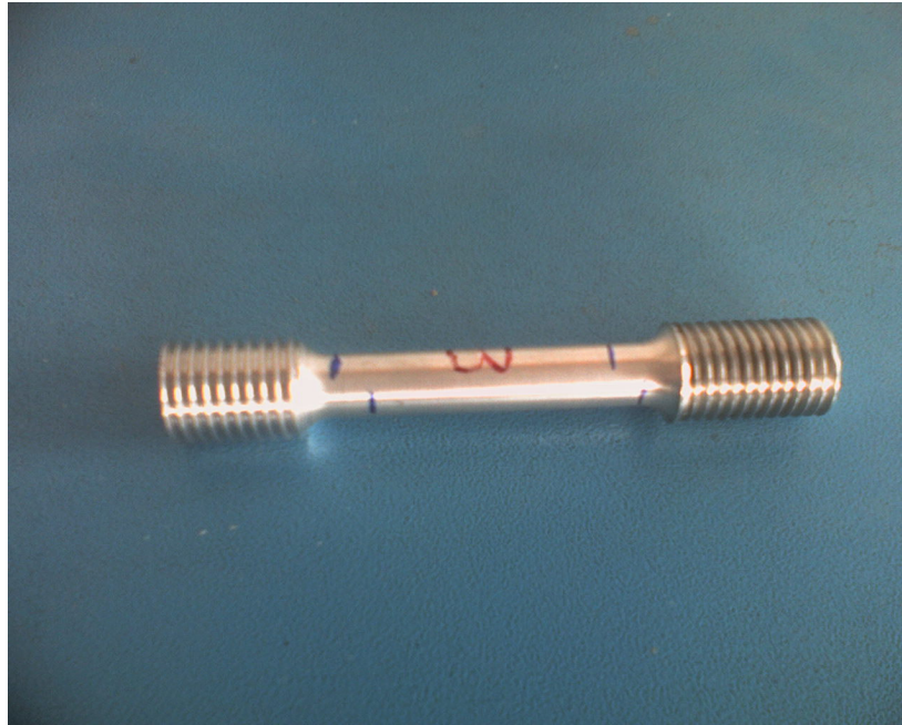
Figure 3.22. Marking and measuring of the initial length ( L_0 ) of the tensile test specimen
