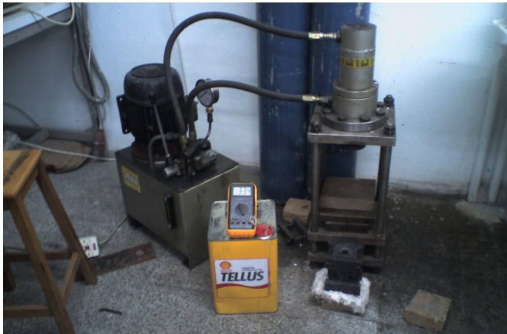
Figure 3.11. The squeeze casting set-up
