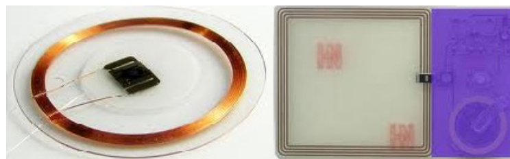
Figure 1.1. Example of passive and active tag.
