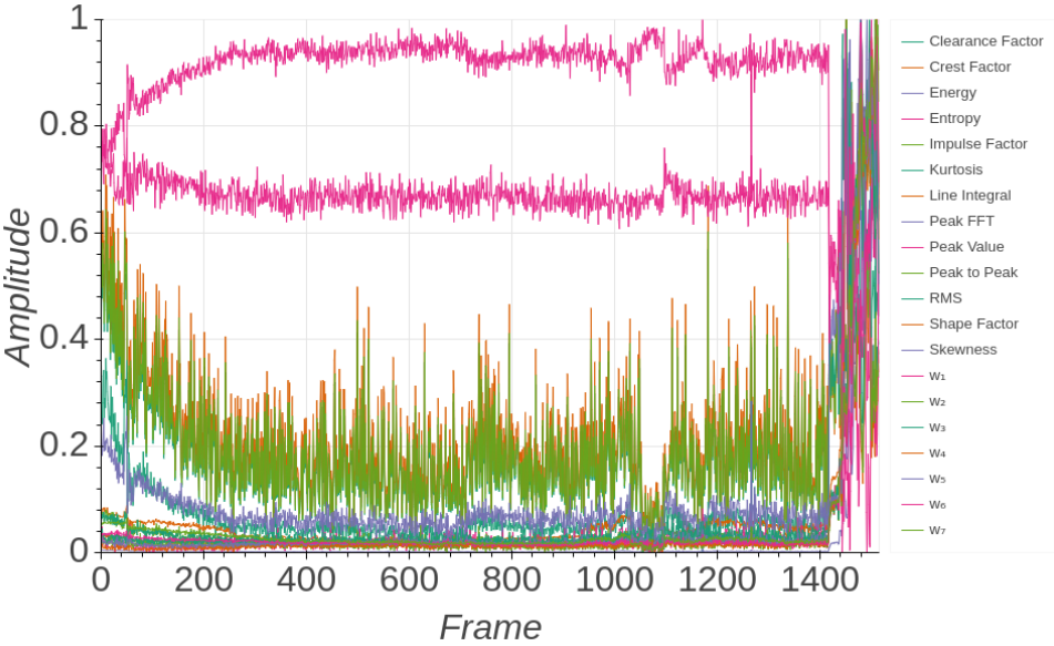
(a) Extracted features from raw vibration signal.
