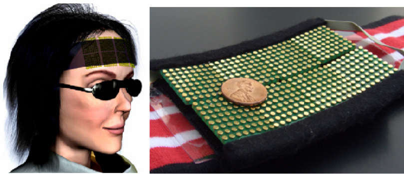
Figure 2.7. 32 \times 16 electrodes module for the forehead [95].
