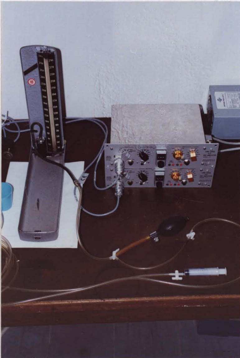
Figure 7.6 Preamplifiers and mercury column manometer set up.
