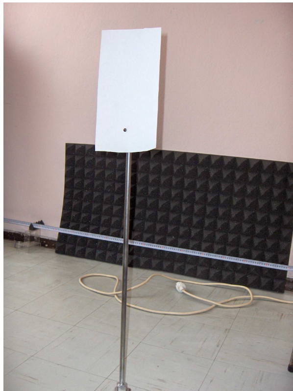
Figure 5.12. The laser beam is projected to a far measuring tape, to increase measurement accuracy
