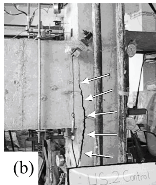
Figure 4.3. Failure modes; (a) pull, (b) push direction of loading
