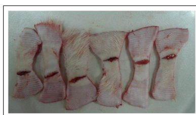
Figure 5.11 Skin samples after tensile strength tests.
