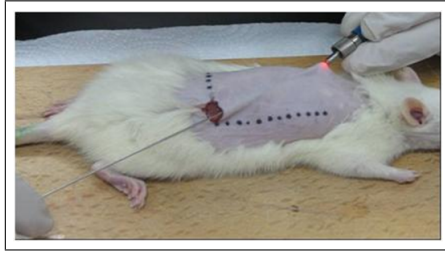
Figure 4.46 Temperature measurements under skin by thermocouples.
