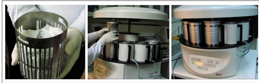
Figure 4.20 Dehydration process by Leica TP1020, Tissue Processor.
