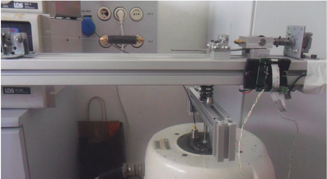
Figure 3.12. The connection of the combined system to the shaker.
