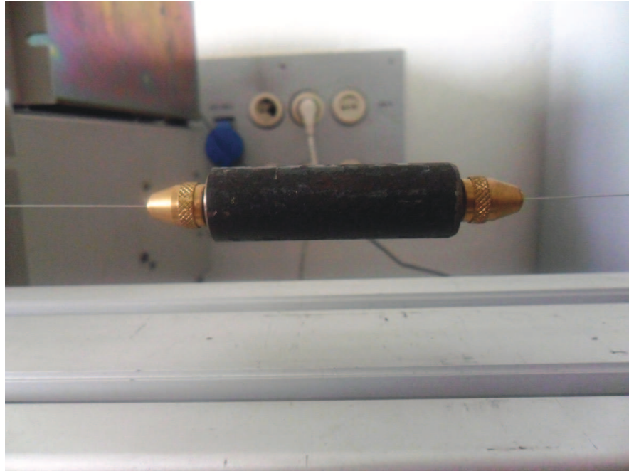
Figure 3.5. Attachment of the mass to the string using drill chucks.
