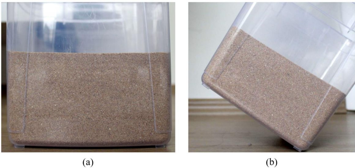
Figure 3.6. Peak Friction Angle Test a) Before and b) After Tilting.
