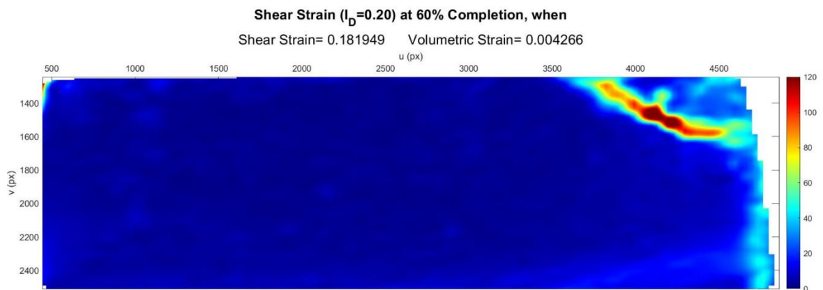
Figure C.23. Shear Strain Field at 60% Completion ( I_D = 0.20 & \sigma' = 0.49 kPa).
