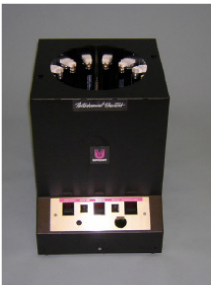
Figure 2.1. Merry-go-round type reactor
