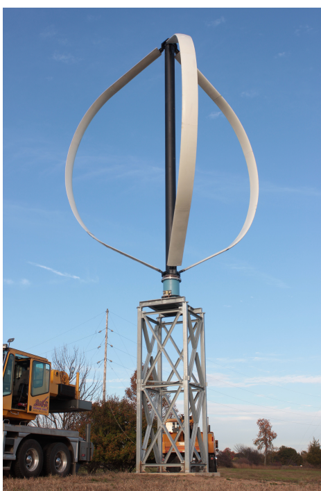
Figure 1.2. Vertical-axis wind turbine (VAW).
