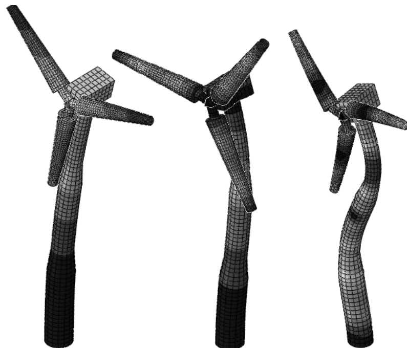
Figure 2.5. First three side-to-side mode shapes obtained in the current study.
