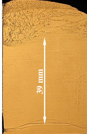
Figure 4.7. The striations and single crystal length of the AVC-20-10-2-0.25.
