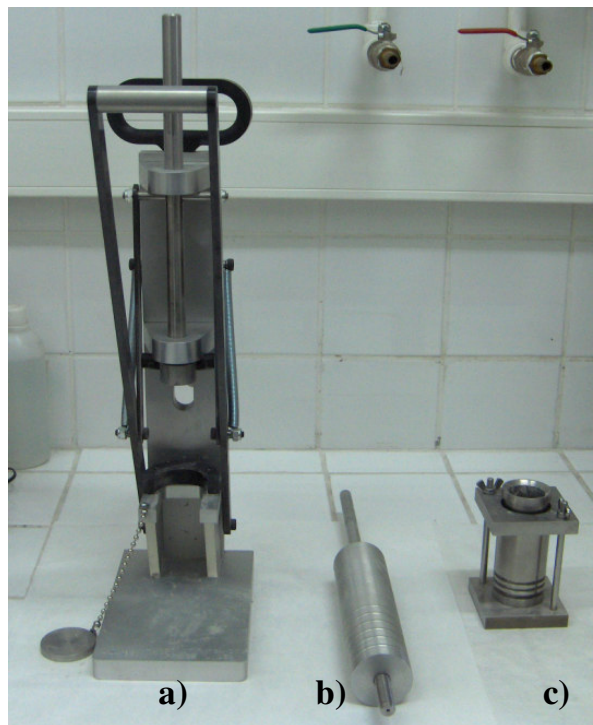
Figure 3.1. Harvard Miniature Compaction Apparatus, a) specimen ejector, b) compaction tamper, c) mold.
