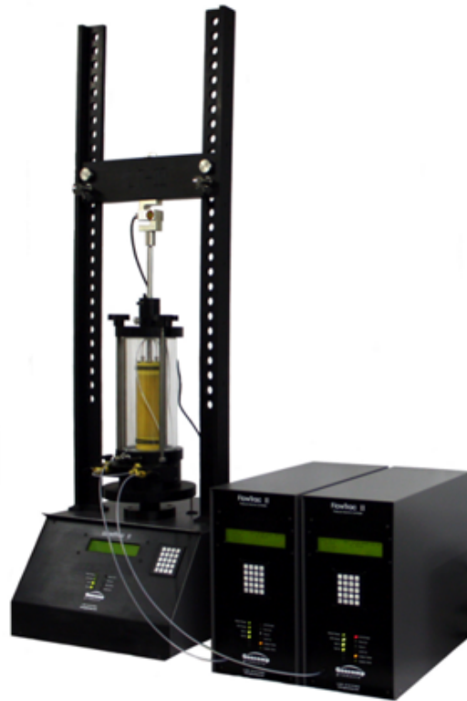
Figure 3.32. Fully Automated Triaxial Testing Apparatus (Abatkon, 2012).
