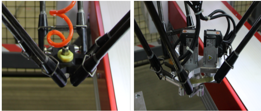
Figure 3.27. The single gripper (left), and the 2-DOF gripper (right) are integrated into the Delta-type manipulator.
