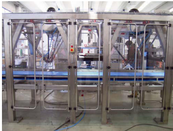
Figure 1.2. Two IRB 360 FlexPicker robots from ABB picking up objects from a conveyor. Reprinted from [15].
