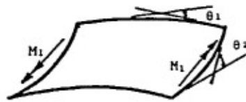
(b) Application of Bending Moment M_1
